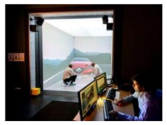
Figure 3. Renault's 70 M 3D pixels 5 – sided high performance CAVE<sup>TM</sup>
