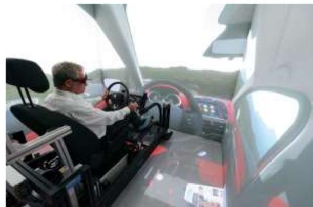
**Figure 5. Renault's high performance CAVE™ with driver station**
