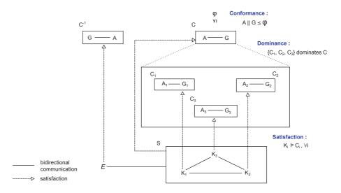
Figure 1: Contract-based reasoning for a subsystem with three components [21].
