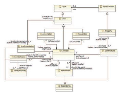
Figure 2: UML meta-model extended with contracts.
