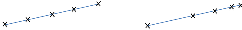
Fig. 1. TSP with uniform speed (left) and deceleration (right). All positions are sampled with the same frequency.
