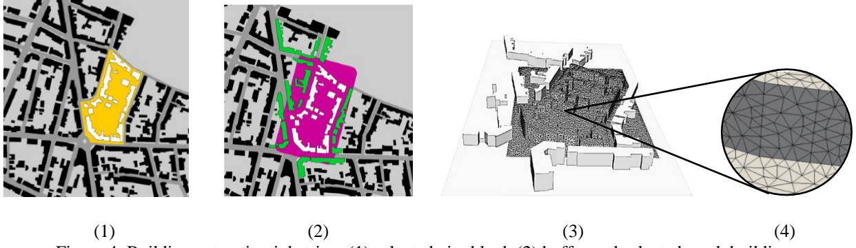
(1) (2) (3) (4) Figure 4. Building extraction jobstring: (1) selected city block (2) buffer and selected mask buildings (3) meshed geometrical model (4) focus on triangular meshes
