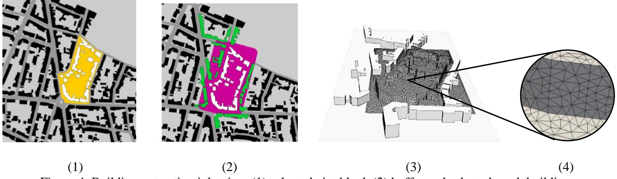
Figure 4. Building extraction jobstring: (1) selected city block (2) buffer and selected mask buildings (3) meshed geometrical model (4) focus on triangular meshes
