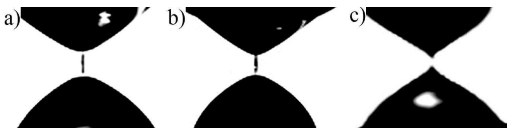
Fig. 3. Evolution of the liquid bridge between two spheres during extension, with constant water volume: (a) Mode 1a (symmetric, two pinchings, volume 4 \mu\text{l} ), (b) Mode 1b (non-symmetric, one pinching, volume 8 \mu\text{l} ), and (c) Mode 2 (rupture in the middle, volume 2 \mu\text{l} ).
