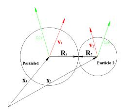
Fig. 1 Velocities of particle 1 and particle 2 in contact
