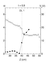
FIG. 3. Spatial evolution of the electronegativity (■) and plasma potential (○) at three different instants during one period of the instability (time normalized to the instability period). Same conditions as Fig. 2.
