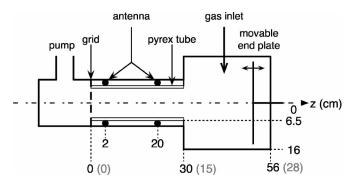
FIG. 1. Schematic of the experimental setup. The dimensions under bracket in gray are that of the corresponding simulation.
