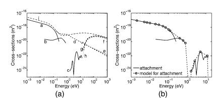
FIG. 5. (a) Electron-neutral collision cross section with  $SF_6$ ; attachment: (a–c); excitations: (d–g); ionizations: (h); elastic collisions: (i). (b) Attachment cross section in  $SF_6$  (solid lines) and simplified total attachment cross-section used in the simulation (broken line).
