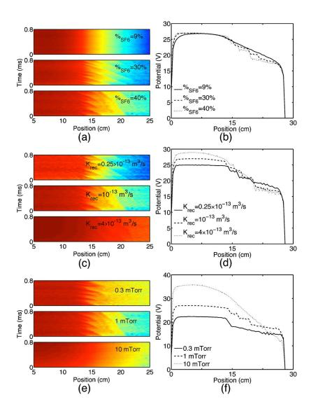
FIG. 7. (Color online) Contour plots of the plasma potential profiles as a function of space and time, and snapshots of the plasma potential profiles, for various relative concentrations of  $SF_6$  [(a) and (b)], recombination rate coefficients [(c) and (d)], and neutral gas pressures [(e) and (f)].
