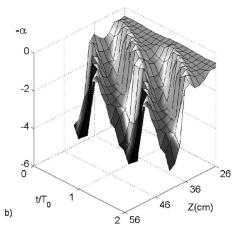
FIG. 2. Spatiotemporal evolution of (a) the plasma potential and (b) the electronegativity in the experimental setup. Time is normalized to the instability period (~850 ms) for a 25% SF<sub>6</sub> concentration plasma at 600 W and 1 mTorr.
