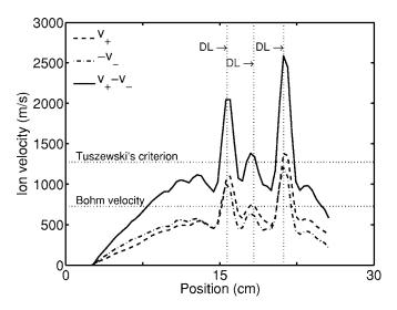
FIG. 10. Snapshot of the positive and negative ion average velocities  $v_+$ ,  $-v_-$  (broken lines) and the relative drift velocity  $v_+$ - $v_-$  (solid line), as a function of position. The vertical dotted lines show the positions of the double layers, while the horizontal lines show the Bohm velocity and "Tuszewski's criterion."
