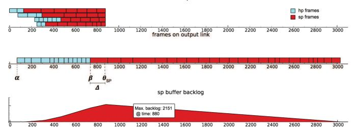
Fig. 1: Intuitive approach for the worst case scenario and computation of the worst case backlog for Buffer<sup>S</sup>.
