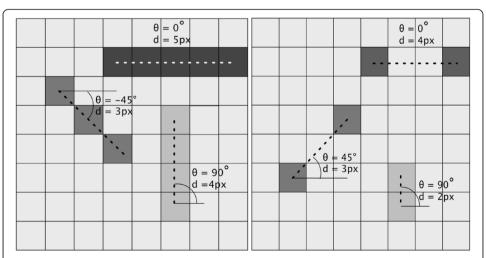
Figure 1 Illustration of the pixel relationship considered by the Run-length matrix approach (left) and the Cooccurrence matrix method (right).
