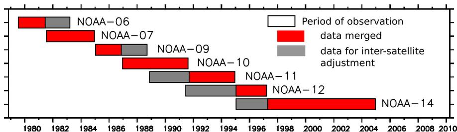
FIG. 3. Satellite observation periods of the NOAA satellites: the red rectangles indicate the data used to merge satellite observations, and the gray rectangles indicate data used to calculate the intersatellite adjustments during overlapping observing periods.
