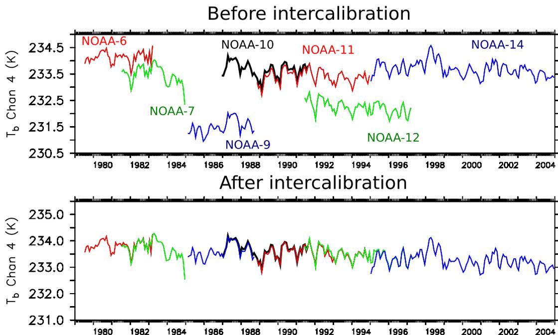
FIG. 4. Clear-sky HIRS brightness temperature  $T_b$  (K) since 1979, averaged between 30°N and 30°S over the ocean, for the 14.2- $\mu$ m channel (channel 4), (top) before and (bottom) after intercalibration.
