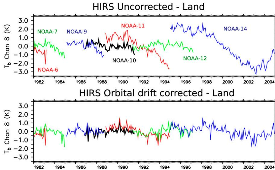
FIG. 1. Clear-sky HIRS brightness temperature  $T_b$  observations (K) since 1979, deseasonalized anomalies, averaged between  $30^{\circ}\text{N}$  and  $30^{\circ}\text{S}$  over land, for the  $11.1\text{-}\mu\text{m}$  window channel (channel 8), (top) using the raw data and (bottom) after orbital drift correction of Jackson and Soden (2007).
