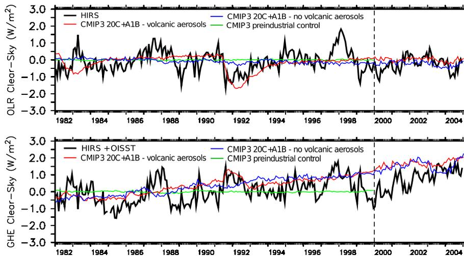
FIG. 12. Time series of clear-sky OLR and GHE ( $\text{W m}^{-2}$ ) deseasonalized anomalies, averaged between  $30^{\circ}\text{N}$  and  $30^{\circ}\text{S}$  over sea surfaces, from HIRS and from the multimodel mean of the coupled models. The results are from the merged 20C/A1B and CTRL simulations. The dashed vertical line indicates the separation between the 20C and A1B simulation periods.
