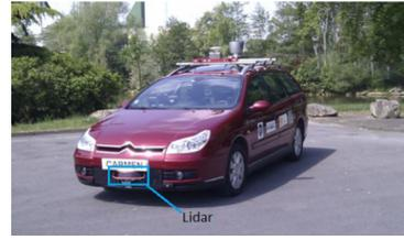
Fig. 1: The LIDAR mounted on the experimental vehicle.
