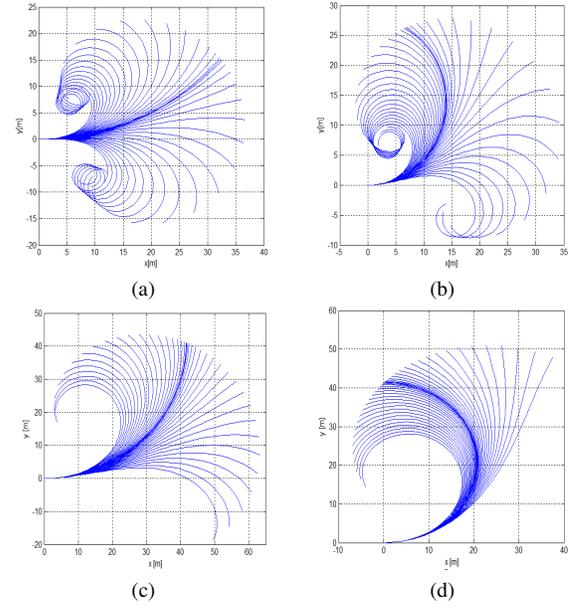
Fig. 3: Different clothoids at different speeds and different initial steering angles: (a)  $V_x=6m/s$   $\delta_0=0.1rad$ , (b)  $V_x=6m/s$   $\delta_0=0.3rad$ , (c)  $V_x=10m/s$   $\delta_0=0.1rad$ , (d)  $V_x=10m/s$   $\delta_0=0.3rad$
