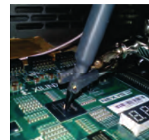
Fig.2: Near Field Probe above FPGA chip
