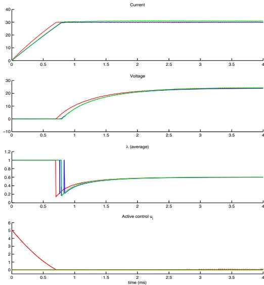
Figure 5. Startup of the Buck-Boost converter (blue: numerical optimal solution ; green: without active control ( $R_i = 10^8$ ); red: with active control ( $R_i = 10^3$ )): time evolution of the voltage, the current, switching control  $\lambda \in [0, 1]$  and of the active control  $u_i$  in presence of measurement noise
