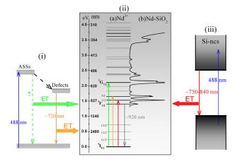
FIG. 12. Schematic illustrations of the  $Nd^{3+}$  ions excitation. (i) Energy diagrams of ASSs and defects within the films annealed at  $T_A\!<\!1000\,^{\circ}C$ , (ii) (a) energy diagram of  $Nd^{3+}$  ions and (b) absorption spectrum of  $Nd^{3+}$  ions doped in  $SiO_2$  film, and (iii) energy diagram of Si-ncs within the films annealed at  $T_A\!>\!1000\,^{\circ}C$ . ET is the abbreviation of energy transfer.
