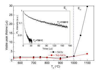
FIG. 10. Evolution of PL lifetimes measured on peak  $E_L$  and  $E_H$  versus  $T_A$  for 1 min-annealed  $SiO_x$  and Nd-SiO $_x$  films detected at the maximum point of each peak. The inset shows the PL decay curves for  $SiO_x$  films annealed at 750 and 1100 °C.
