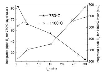
FIG. 3.  $E_L$  and  $E_H$  peak intensity versus  $t_A$  for  $SiO_x$  films annealed at 750 °C (left scale) and 1100 °C (right scale), respectively.
