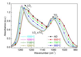
FIG. 5. FTIR spectra recorded at Brewster angle of  $65^{\circ}$  for  $\text{SiO}_x$  films deposited on a Si wafer and annealed at indicated  $T_A$  during 1 min. The spectra were normalized with respect to the  $TO_3$  band intensity.
