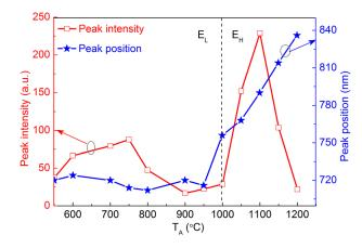
FIG. 2. Peak intensity (left scale) and position (right scale) of SiO<sub>x</sub> films versus T<sub>A</sub>.
