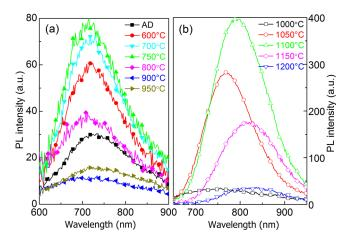
FIG. 1. The PL spectra of SiO<sub>x</sub> films annealed at the indicative temperature with 1 min duration. The left (a) corresponds to T<sub>A</sub> lower than 1000 °C while the right (b) to high T<sub>A</sub> higher than 1000 °C. AD is the abbreviation of as-deposited.
