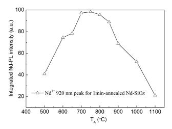
FIG. 9. Evolution of  $Nd^{3+}$  PL intensity as a function of  $T_A$  for  $Nd\text{-}SiO_x$  films annealed during 1 min.
