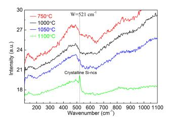
FIG. 4. RAMAN spectra of the  $SiO_x$  films deposited on quartz substrate and annealed at indicated  $T_A$  for 1 min.
