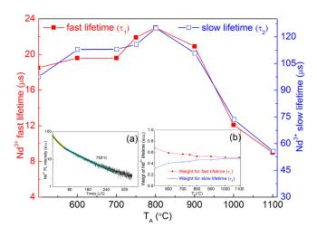
FIG. 11. Evolution of  $Nd^{3+}$  PL lifetime at 920 nm versus  $T_A$ . The inset (a) is a representative decay rate of  $750\,^{\circ}$ C  $Nd\text{-SiO}_x$  PL, fitted by a two-exponential decay model, while the inset (b) is the component of  $Nd^{3+}$  fast or slow lifetime.
