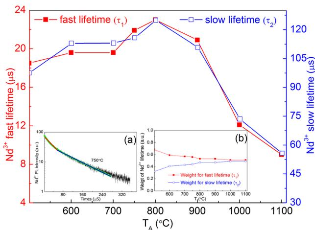
FIG. 11. Evolution of  $\text{Nd}^{3+}$  PL lifetime at 920 nm versus  $T_A$ . The inset (a) is a representative decay rate of  $750^\circ\text{C}$   $\text{Nd-SiO}_x$  PL, fitted by a two-exponential decay model, while the inset (b) is the component of  $\text{Nd}^{3+}$  fast or slow lifetime.
