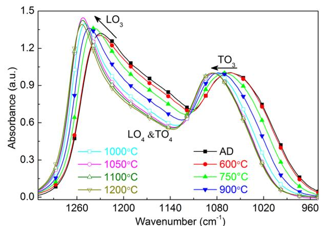
FIG. 5. FTIR spectra recorded at Brewster angle of 65° for  $\text{SiO}_x$  films deposited on a Si wafer and annealed at indicated  $T_A$  during 1 min. The spectra were normalized with respect to the  $\text{TO}_3$  band intensity.
