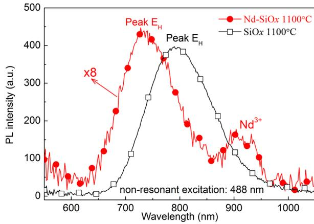
FIG. 8. PL spectra of Nd-SiO<sub>x</sub> and SiO<sub>x</sub> films annealed for 1 min at 1100 °C.
