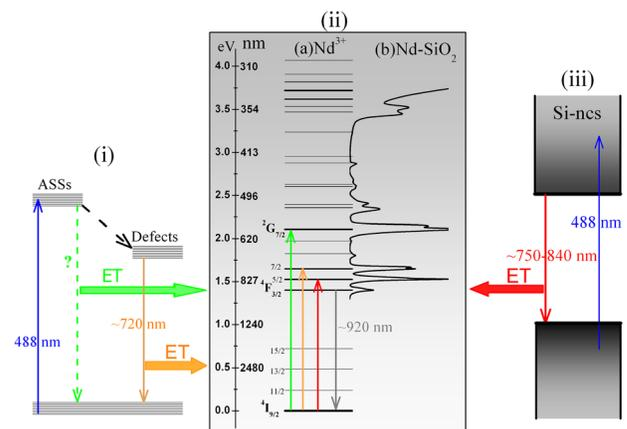
FIG. 12. Schematic illustrations of the  $\text{Nd}^{3+}$  ions excitation. (i) Energy diagrams of ASSs and defects within the films annealed at  $T_A < 1000^\circ\text{C}$ , (ii) (a) energy diagram of  $\text{Nd}^{3+}$  ions and (b) absorption spectrum of  $\text{Nd}^{3+}$  ions doped in  $\text{SiO}_2$  film, and (iii) energy diagram of Si-ncs within the films annealed at  $T_A > 1000^\circ\text{C}$ . ET is the abbreviation of energy transfer.
