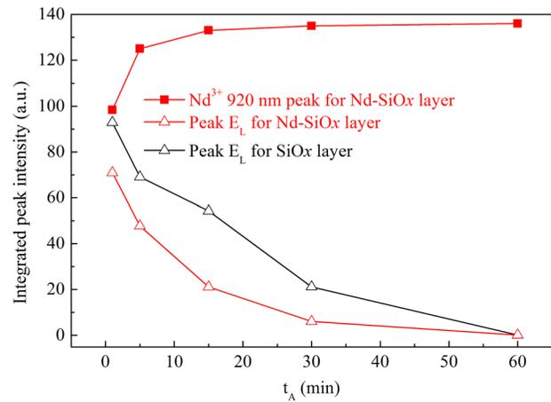
FIG. 7. Integrated peak intensities of Nd-SiO<sub>x</sub> and SiO<sub>x</sub> films annealed at 750 °C versus t<sub>A</sub>.
