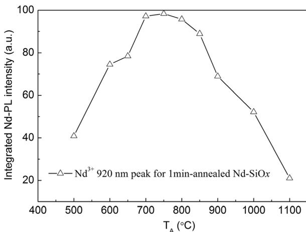
FIG. 9. Evolution of Nd<sup>3+</sup> PL intensity as a function of  $T_A$  for Nd-SiO<sub>x</sub> films annealed during 1 min.
