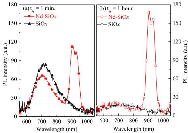
FIG. 6. PL spectra of Nd-SiO<sub>x</sub> and SiO<sub>x</sub> films annealed at 750 °C during (a) 1 min and (b) 1 h.
