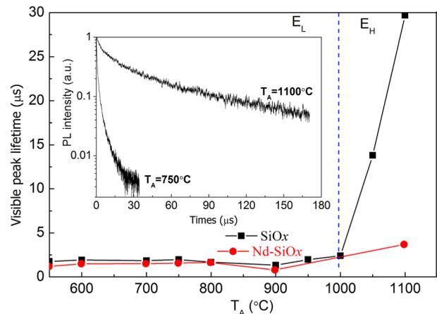
FIG. 10. Evolution of PL lifetimes measured on peak E<sub>L</sub> and E<sub>H</sub> versus  $T_A$  for 1 min-annealed SiO<sub>x</sub> and Nd-SiO<sub>x</sub> films detected at the maximum point of each peak. The inset shows the PL decay curves for SiO<sub>x</sub> films annealed at 750 and 1100 °C.
