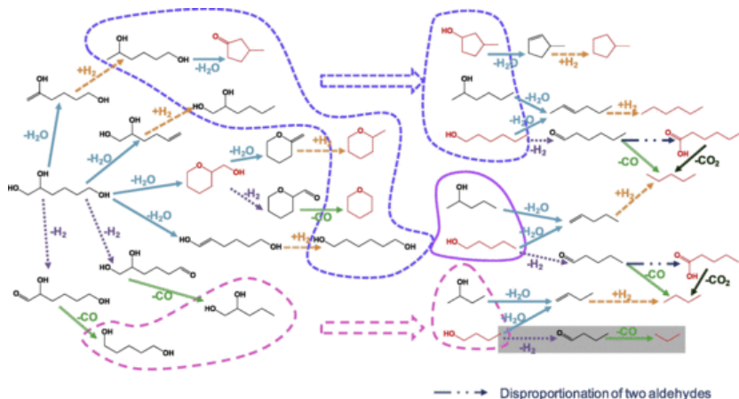
Fig. 9 Reaction scheme of 1,2,6-hexanetriol transformation over Pt/ZrO 2 + TiO 2 -WO x .
