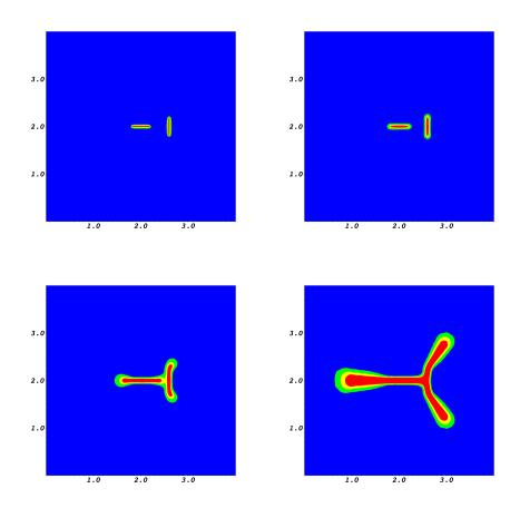
Figure 7: Example 3: Crack pattern (in red with  $\varphi = 0$ ) for four different time steps at T = 1, 25, 30, 35. The unbroken material is denoted in blue with  $\varphi = 1$ . The mushy zone is yellow/green.
