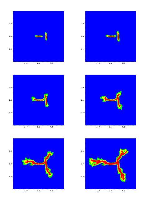
Figure 9: Example 4: Crack pattern (in red with  $\varphi=0$ ): joining, branching and non-planar crack growth in a heterogeneous medium. The unbroken material is denoted in blue with  $\varphi=1$ . The mushy zone is yellow/green.
