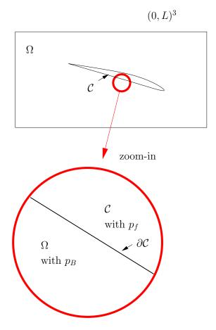
Figure 1: Configuration and notation of the reservoir domain  $\Omega$  and the crack  $\mathcal{C}$  and zoom-in to the crack boundary  $\partial \mathcal{C}$  where the interface law (7) is prescribed. We recall that  $\Omega = (0, L)^3 \setminus \overline{\mathcal{C}}$  and  $\partial \Omega = \partial (0, L)^3 \cup \partial \mathcal{C}$ .
