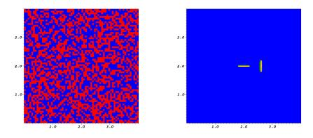
Figure 8: Example 4:  $\mu$ -distribution (left) and initial crack configuration (right). The Lamé parameter  $\mu$  varies in a range of 0.42-1.41 where the red parts denotes stiff material and the blue regions smoother material.
