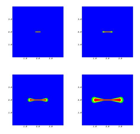
Figure 4: Example 2: Crack pattern (in red with  $\varphi=0$ ) for four different time steps at T=1,30,35,40. The unbroken material is denoted in blue with  $\varphi=1$ . The mushy zone is yellow/green.
