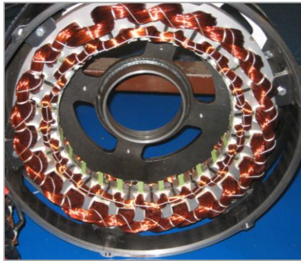
Fig.3b: Picture of stator of the HEFSSM prototype 24-20.
