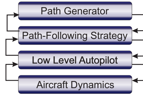
Fig. 9. Communication scheme between the MAV3DSim and the CRRC-Sim.
