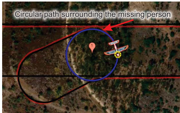
Fig. 11. Circular path generated to surround the missing person.
