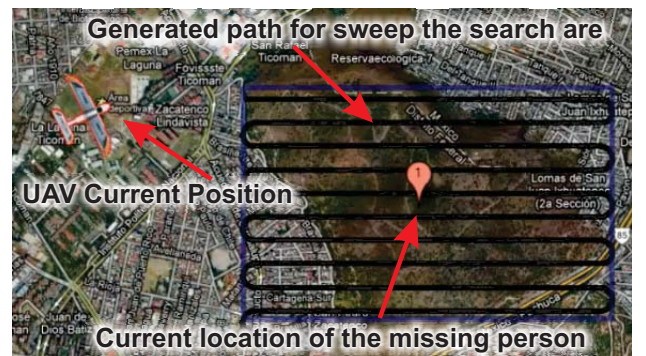
Fig. 10. The path generated to weep the search area.
