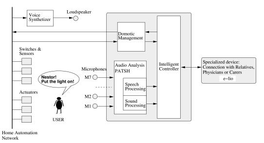
Figure 1: The SWEET-HOME system: example of a user asking to switch the light on.
