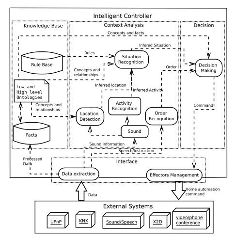
Figure 4: The Intelligent Controller Diagram.
