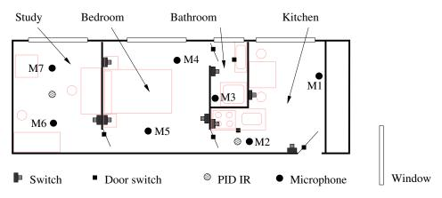
Figure 6: Position of the microphones and other sensors inside the DOMUS smart home.
