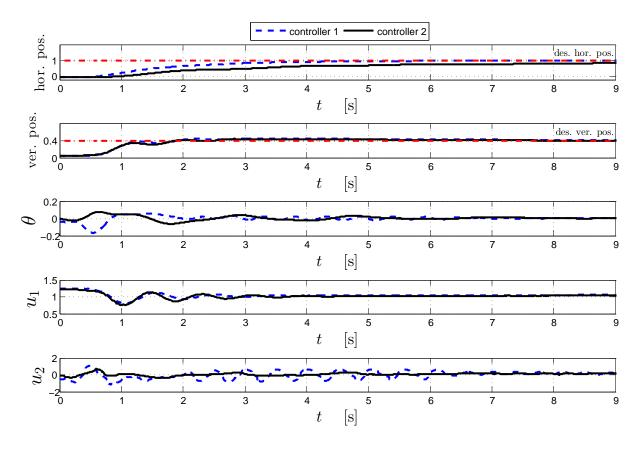
Fig. 3. Experimental results: position responses (horizontal, vertical,  $\theta$ ) and control signals ( $u_1, u_2$ ).
