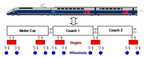
Figure 2: Simplified description of a multibody model of a TGV.
