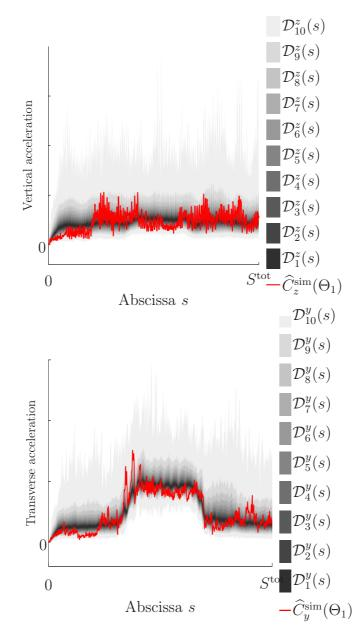
Figure 7: Influence of the track variability on the maximal values of the accelerations in the train coaches.
