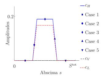
Figure 3: Evolution of the horizontal curvature  $c_H$  (× $km^{-1}$ ), the vertical curvature  $c_V$  (× $km^{-1}$ ) and of the cross level  $c_L$  (× $m^{-1}$ ) with respect to the track curvilinear abscissa s.
