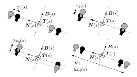
Figure 1: Parametrization of the track irregularities, where E the theoretical track gauge, s is the curvilinear abscissa of the track and  $(O_{NT}(s), T(s), N(s), B(s))$  is the Frenet frame (for each rail, the mean position is represented in black, whereas the real position is in grey).
