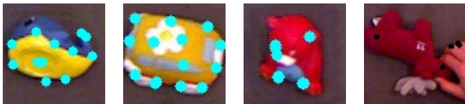
Fig. 3. Example frames from the image dataset. This frames feature the following objects: blue whale , yellow car , teddy bear and moose . Color circles corresponds to local descriptors detected by the system. Interestingly, the hand of the operator appears in some pictures as in the last one. The area observed by the system is actually larger than the one represented in the figure.
