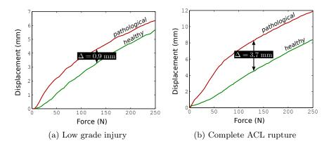
Figure 3: Response curves as given by the  $GNRB^{\textcircled{R}}$  device: (a) partial tear with differential laxity of 0.9 mm at 134 N (subject 5); (b) complete ACL rupture with differential laxity of 3.7 mm at 134 N (subject 11).
