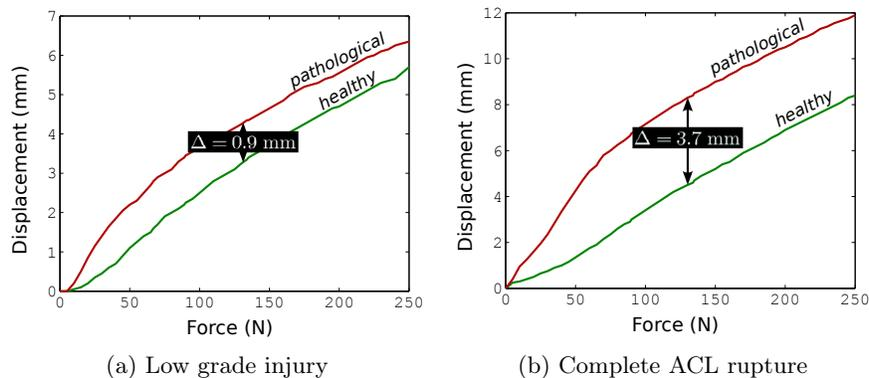
Figure 3: Response curves as given by the GNRB<sup>®</sup> device: (a) partial tear with differential laxity of 0.9 mm at 134 N (subject 5); (b) complete ACL rupture with differential laxity of 3.7 mm at 134 N (subject 11).
