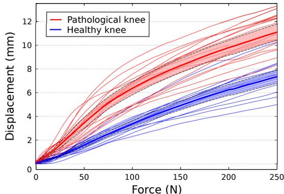
Figure 6: Displacement-load test curves given by the GNRB<sup>®</sup> arthrometer of healthy and pathological knees for the 16 subjects. Bold lines represent the means and dashed lines the 95% CIs for the means.
