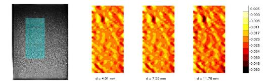
Figure 7: ROI calculated in quasi-static loading and the longitudinal strain fields
