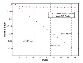
Figure 8: Comparison of the global nominal strain and the mean local strain in the quasi-static loading
