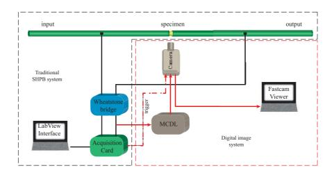
Figure 10: Diagram of SHPB system and the digital image photography system
