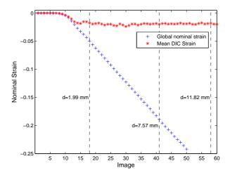
Figure 15: Comparison of the global nominal strain and the mean local strain in the dynamic loading
