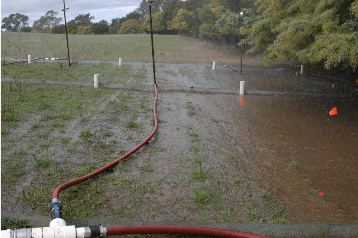
Figure 3 A view towards the South, over the experimental site, showing Plot I (foreground) and Plot II (middle distance) during the first simulated rainfall event (48 mm/h). Water is beginning to pond on the pasture (left) and bare soil area (right) is generating overland flow, which is draining onto the tree belt (far right). A small backwater can be seen extending about 1 m uphill from the fence on the far plot (plot II).
