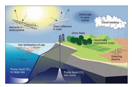
Fig. 7. Schematic representation of various climate-engineering proposals (Keith 2001). It is essential that numerical experimentation with high-resolution weather, climate, and complex Earth system models, with established fidelity and skill, provide scientifically based assessments of the global to regional impact of such engineering hypotheses prior to their design and implementation.
