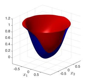
Figure 2: Nonlinear double integrator – upper bound on the value function  $\overline{V_u}$  associated to the extracted controller (red); lower bound on the optimal value function  $\underline{V}$  (blue).
