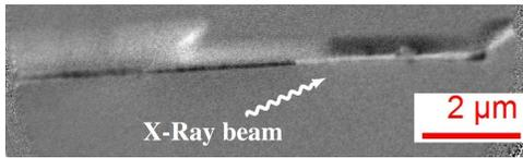
Fig. 4. XMCD image of a trisegmented nanowire and its shadow. There is an angle of  $\sim 30^\circ$  between the X-ray beam and the wire. A DW is pinned in the thin middle section of the wire, as shown by the abrupt contrast change.
