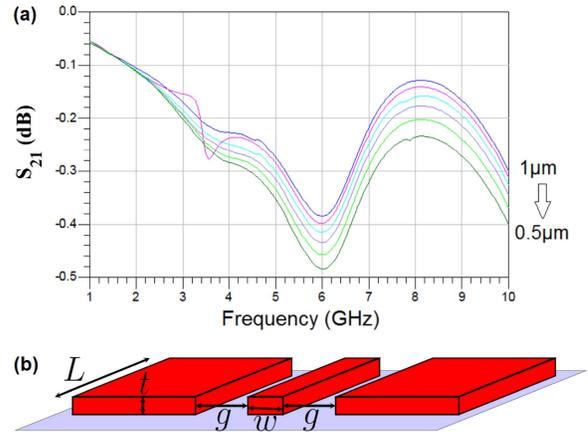
Fig. 2. (a) Simulations of a CPW with length  $L = 2.5$  cm, central track width  $w = 0.65$  mm, gap  $g = 0.25$  mm, and varying thickness  $t$ . (b) Schematics of a CPW with the definition of  $t$ ,  $w$ ,  $L$ , and  $g$ .
