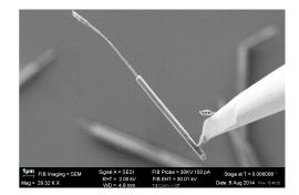
Fig. 3. FIB-assisted nanowire micromanipulation. The manipulating tip on the right barely contacts the wire, which has been lifted up off its substrate. Here, one of this wire's thick parts was broken during dispersion.
