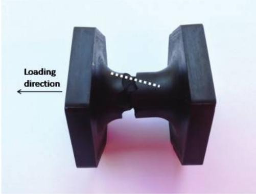
Figure 4. Direction of the crack propagation plane.
