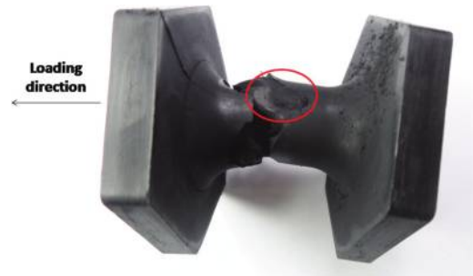
Figure 6. Ruptured dry specimen.
