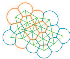
Figure 4: Adhesive forces are simulated with springs that connect cells centers, allowing for the formation of compact cellular clusters of various stiffnesses.
