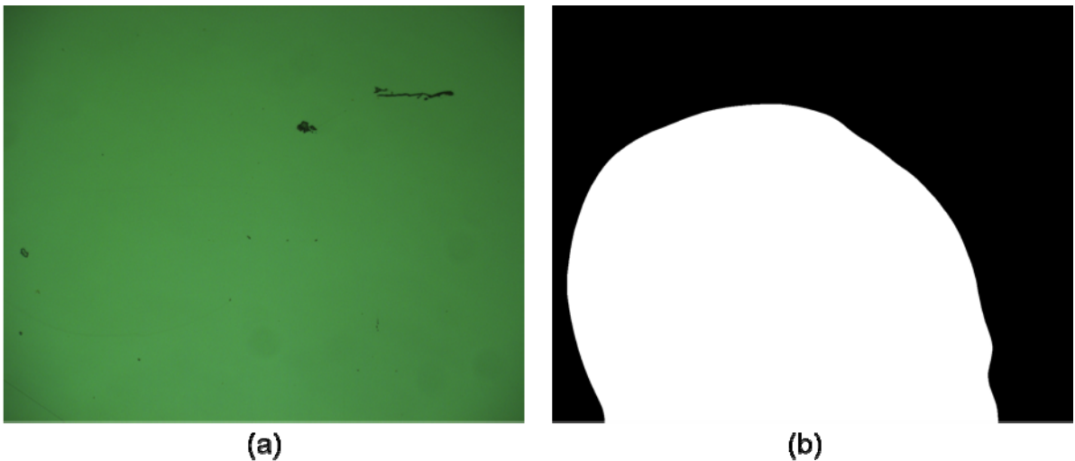
Figure 3. (a) Non-uniform irradiance on a sample from the learning set consisting of a ROSCO green filter on top of the calibrated mirror. (b) Area considered for the average color extraction of the samples in the learning set consisting of ROSCO color filters on top of the calibrated mirror. The area corresponds to pixels with color difference lower than 5 CIE-DeltaE94 units with respect to the pixel with the highest CIELAB L^* value.
