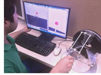
Fig. 4: A picture of the experimental setup. The human operator teleoperates the UAV using the haptic device and relies on a fixed camera (left) and an onboard camera (right) to see the virtual environment.
