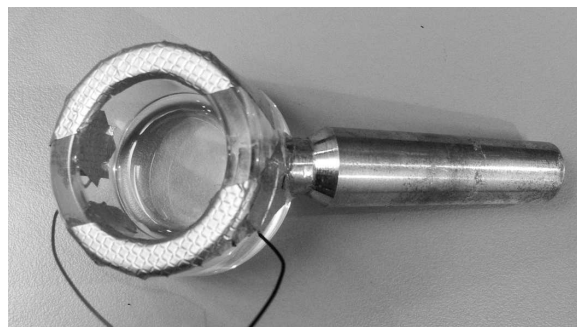
Figure 2. (a) Schematic description of an EGG device. (b) Transparent mouthpiece developed by Castellango et al. [40] equipped with copper foil shielding tape electrodes.
