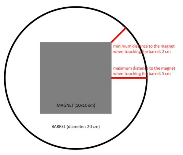
**ESM Fig. 2** Sketch of the barrel containing the neodymium block (view from above). When touching the barrel, the distance to the magnet is 2-5 cm depending on the position.
