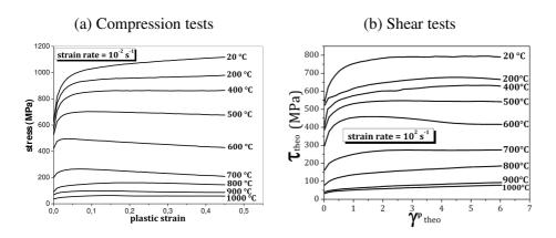
Figure 2: Evolution of (a) the compressive stress as a function of the plastic strain at a strain rate of  $10^{-2} s^{-1}$  and (b) the shear stress as a function of the plastic shear strain at an equivalent strain rate of  $10^2 s^{-1}$  for the 42CrMo4-BA steel.
