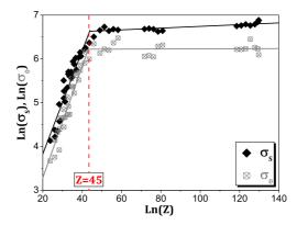
Figure 11: Experimental values and linear regression parameters ( $\sigma_s$  and  $\sigma_0$ ) for the Lurdos model for the 42CrMo4-BA steel.
