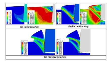
Figure 16: Description of the chip formation process in the numerical simulation.
