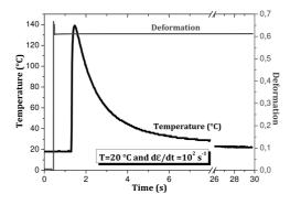
Figure 4: Experimental measurement of the temperature increase during compression deformation of the 42CrMo4-BA steel at  $T = 20^{\circ}C$  and  $\dot{\varepsilon} = 10^2 s^{-1}$  (Hor et al. (2013)).
