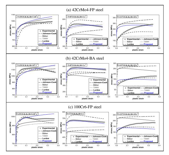
Figure 12: Comparison between the different constitutive models for different thermomechanical conditions for the three steels investigated: (a) 42CrMo4-FP, (b) 42CrMo4-BA and (c) 100Cr6-FP.
