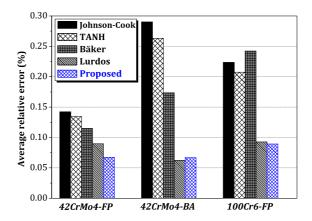
Figure 13: Average relative error between the experimental results and the predictions of the different constitutive laws identified for the three steels investigated. The proposed model is shown in blue.
