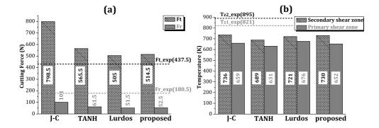
Figure 18: Comparison between the cutting forces (on the left) and the temperatures (on the right) obtained via numerical simulation using different constitutive models and corresponding experimental observations for the cutting conditions:  $V_c = 250 m/min$  and f = 0.2 mm/rev.
