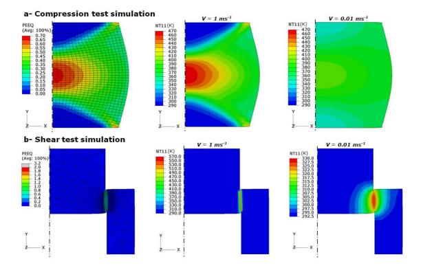
Figure 5: Self-heating temperature fields obtained by numerical simulation of the (a) compression and (b) shear tests for two speeds (1 and  $10^{-2} m s^{-1}$ ).
