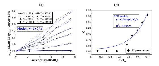
Figure 8: (a) Identification of the various parameters  $C_i$  related to different temperatures  $T_i$  and (b) correlation between the function C(T) and the parameters  $C_i$ , for the 42CrMo4-BA steel.
