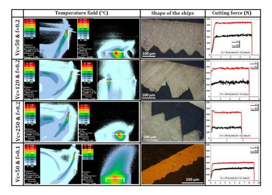
Figure 14: Evolution of the temperature field (°C), the cutting force (N), and the chip shape as a function of the feed rate (mm/rev) and the cutting speed (m/min) for the machining of the 42CrMo4-BA steel.
