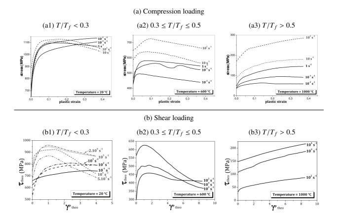
Figure 3: Evolution of (a) the compressive stress as a function of the plastic strain and (b) the shear stress as a function of the plastic shear strain, at  $20^{\circ}C$ ,  $600^{\circ}C$  and  $1000^{\circ}C$ , for different equivalent strain rates for the 42CrMo4-BA steel.
