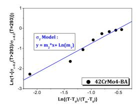
Figure 7: Identification of the parameters  $m_1$  and  $m_2$  from experimental database for the 42CrMo4-BA steel.
