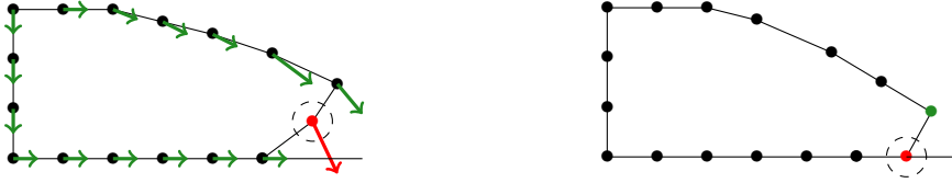
Figure 2: Case when a free surface node goes to the bottom for the configuration (b) with rigid bed. (Left) Dots represent the boundary nodes at time t^n . The arrows represent the displacement \Delta t \mathbf{w}_h^n that comes in (3.1), before limitation of the time step. (Right) New position of the nodes at time t^{n+1} . The time step has been diminished so that no boundary node crosses the bottom. In the illustrated situation, one node that was on the free surface at time t^n is now at the bottom boundary, and one boundary element that was part of the free surface is now part of the bottom. In our simulations of configuration (b) with rigid bed, the effective change of nature of a part of the free surface occurs at most twice between initial and final time.
