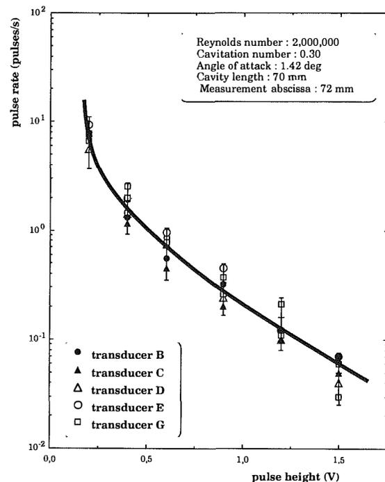
Fig. 2 In-situ relative calibration of 5 pressure transducers
