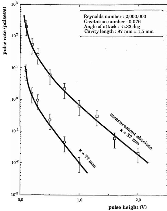
Fig. 3 Pressure pulse height spectra at different abscissa (cavitation number: 0.076)
