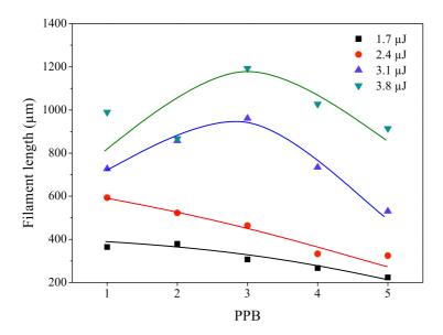
Figure 7. Measurement of the filament length according to experiments in loose focusing configuration and dynamic mode reported on figure 6 with respect to the number of PPB, at 500 kHz. The data are underlined with spline fits.
