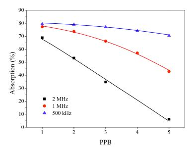
Figure 4. Absorption efficiency of the intravolume interaction versus the number of PPB. The measurements were done in dynamic configuration at 5 mm·s<sup>-1</sup>. The average power available on target was 500 mW for each repetition rate. The target pulse energy was 0.25, 0.5, 1 and 2  $\mu$ J for 2 MHz, 1MHz, 500 kHz and 250 kHz respectively. The data are underlined with spline fits.
