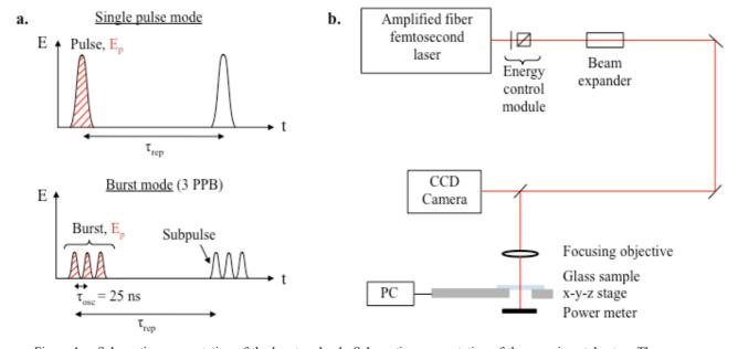
Figure 1. a Schematic representation of the burstmode.. b. Schematic representation of the experimental setup. The energy control module is composed of a half-wave plate and a polarizing beam splitter cube.
