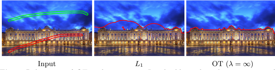
Fig. 2. Robustness of OT with respect to L_1 : the blue colors that are not in the reference histograms are considered as background with OT distance and as foreground with the L_1 model, since no color transport is taken into account.
