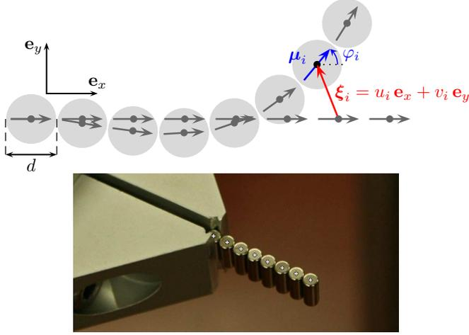
Fig. 1: Top: Sketch of a chain of magnetic dipoles at equilibrium and deformed configurations (here,  $n = 8$ ). Bottom: Photography of the experimental setup. The clamped is realized using aluminium triangles.
