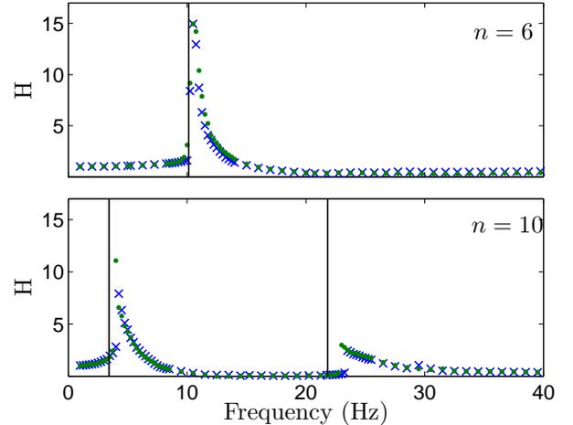
Fig. 4: Modulus of the transfer function between displacement of the clamped cylinder and the cylinder at 3/4 of the length of the chain. Each mark corresponds to an average over 20 seconds. The ( $\times$ ,  $\cdot$ ) symbols represent the up and down sweep direction respectively. The vertical lines are the linear eigenfrequencies predicted by the model.
