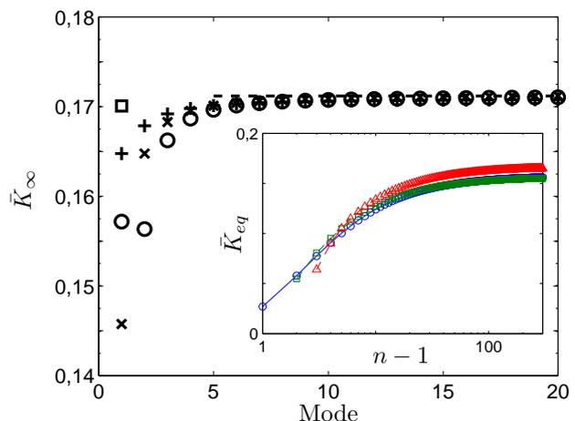
Fig. 6: Normalized equivalent bending rigidity for  $n \rightarrow \infty$  as function of the mode number; (o), clamped-free boundary conditions; ( $\times$ ), pinned-pinned boundary conditions; (+), clamped-clamped boundary conditions; (---), value predicted in reference [6] for a ring. Inset : Equivalent bending rigidity normalized by  $\mu_0 m^2 / \pi D^2$  as function of  $n - 1$ ; (o), mode 1; ( $\square$ ), mode 2; ( $\Delta$ ); mode 3.
