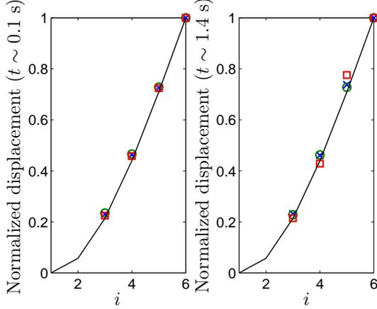
Fig. 3: (—), first theoretical eigenmode for  $n = 6$ , normalized by the displacement of the  $n^{\text{th}}$  dipole; ( $\times$ ,  $\square$ ,  $\circ$ ), displacement of each individual cylinder measured when the chain reaches a maximum of displacement. Left:  $t \sim 0.1$  s, *i.e.* second maximum of Fig. 2(top). Right: maximum of displacement around  $t \sim 1.4$  s, after 17 oscillations. Both times are marked by vertical lines in the top of Fig. 2.
