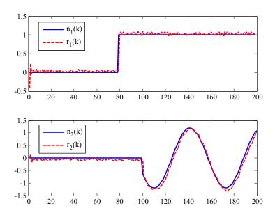
Figure 2: The fault estimation result of the proposed filter
