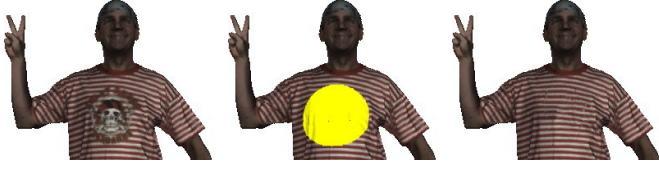
Fig. 1: Real object (with 127,039 points) inpainting with k_G = 30000 and n^2 = 81 . From left to right respectively: the original man, the part to be inpainted shown in yellow, the inpainted man.
