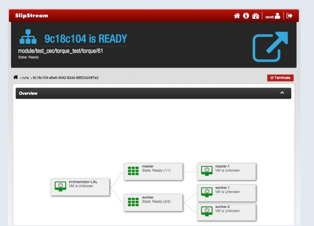
SlipStream Web interface: example of Torque deployment on a virtual cluster of one master node and two worker nodes.
